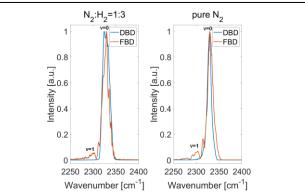
**Fig. 1**. Averaged  $N_2$  vibrational CARS spectra of FBD and DBD in pure  $N_2$  and  $N_2/H_2$  mixture.
